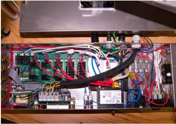
3 Gp, Feb 2006: SPF relays on zones 4 & 5 on 3 gp machines, 2a transformer fuses, 16a pump reset fuses on 3 gp only
